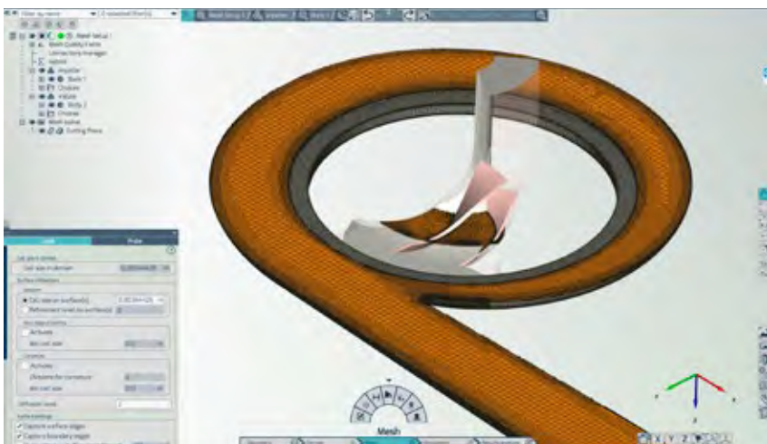
FIGURE 5 : Combined structured mesh impeller (AutoGrid5™) and unstructured mesh volute (HEXPRESS™) of a turbocharger
