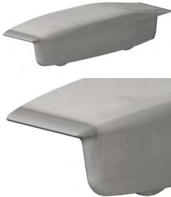
FIGURE 3 : Front view of the mesh generated by HEXPRESS™/Hybrid
