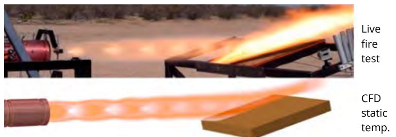
FIGURE 1 : Plume impingement test. Comparison of a photograph and the simulated static temperature
