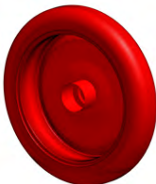
FIGURE 6 : Full hexahedral mesh on the tire surface
