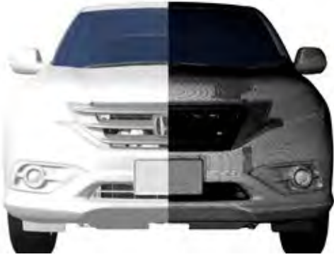
FIGURE 3 : Geometry (left) and its surface mesh (right) of the CR-V model
