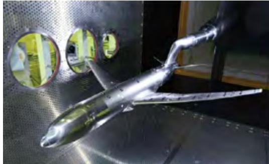
FIGURE 1 : 80% scaled copy of the CRM was performed in the 2m × 2m transonic wind tunnel of JAXA. Spanwise wing sections distribution.
