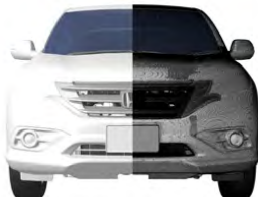
FIGURE 1 : Combined view of geometry and mesh of Honda CR-V model
