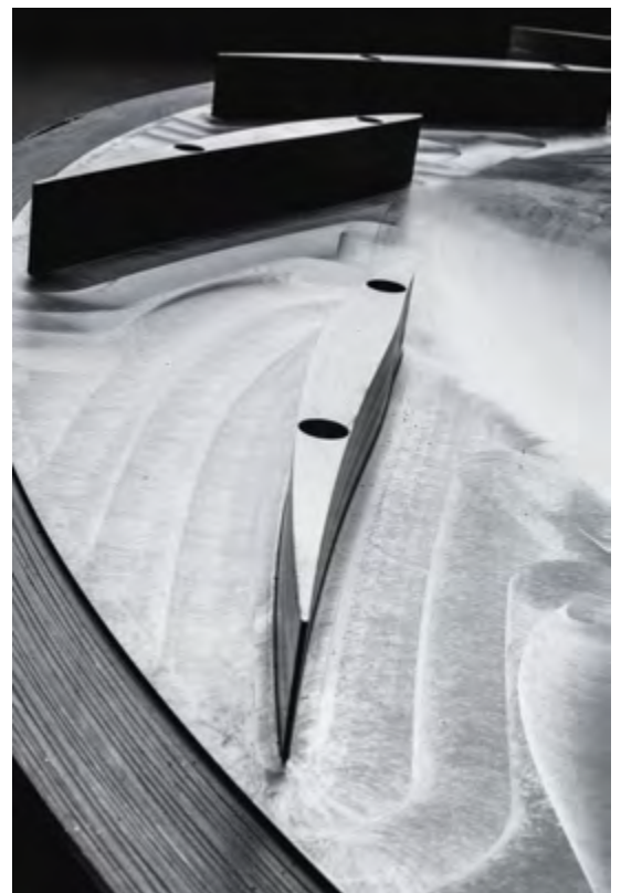
FIGURE 2 : Low density vane diffuser
