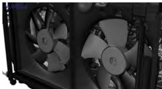
FIGURE 3 : Counter-rotating fans in front of radiator and condenser
